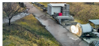
Sequence of a metal dust explosion: conventional explosion venting with an explosion vent.
