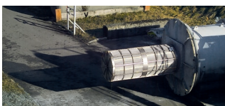
Identical explosion with the Q-Rohr®: no heat generated outside the vessel with only a slight pressure rise and minimal noise volume.
