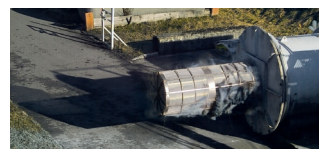
Identical explosion with the Q-Rohr®: no heat generated outside the vessel with only a slight pressure rise and minimal noise volume.
