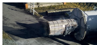
Identical explosion with the Q-Rohr®: no heat generated outside the vessel with only a slight pressure rise and minimal noise volume.
